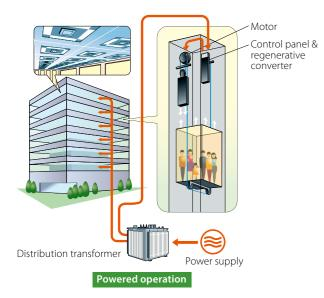
network in the building along with electricity from the power supply. Compared to the same type of elevator without a regenerative converter, this system provides an energy-saving effect of approximately 35%.\* In addition, the regenerative converter has the effect of decreasing harmonic currents.
